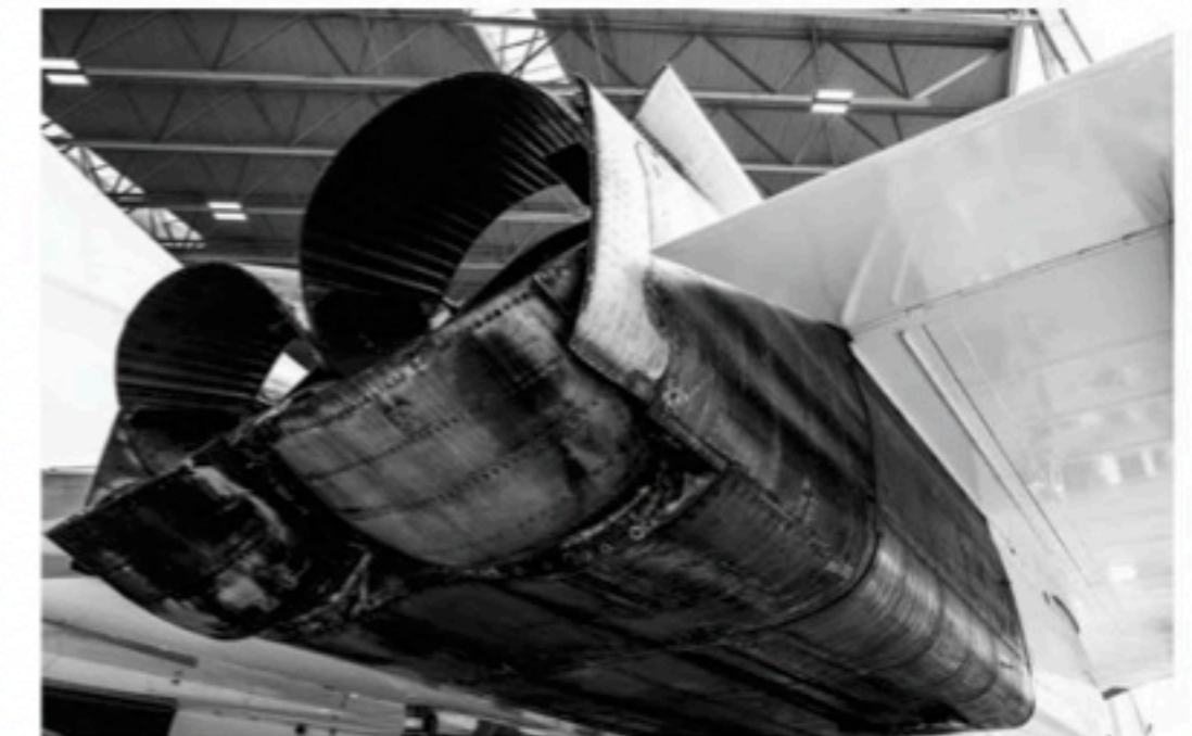
Concorde's secondary engine nozzle featured a hinged-bucket or clamshell design used to efficiently direct exhaust and serve as a thrust reverser to aid deceleration in flight and upon landing.
