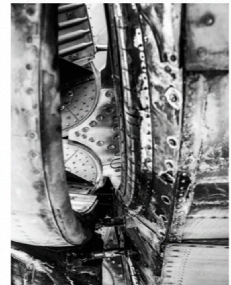
Concorde's secondary engine nozzle featured a hinged-bucket or clamshell design used to efficiently direct exhaust and serve as a thrust reverser to aid deceleration in flight and upon landing.
