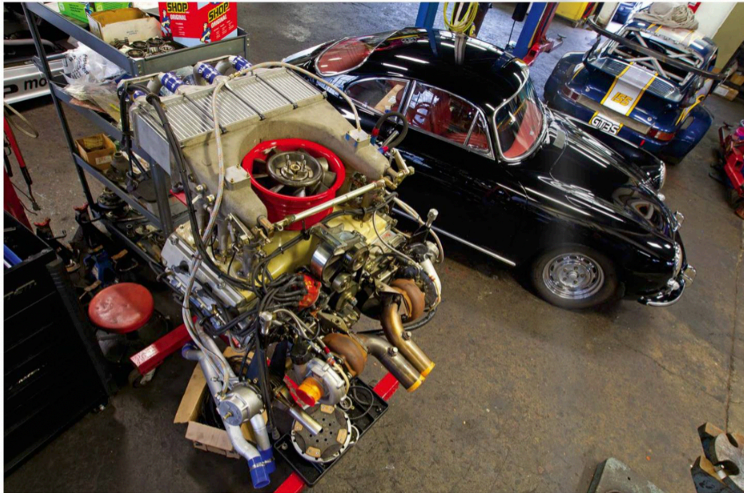
Rebuilding the engine from a Porsche 935 would be a rare feat for many shops, but it's just another day for Dawe's crew.
